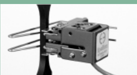
3442 with 6 mm gage length and ±10% gage range.
