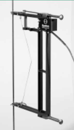
3542L with 8 inch gage length and ±0.4 inches measuring range.
