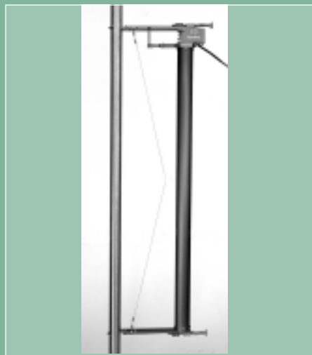
3542L with 500 mm gage length and ±10 mm measuring range.
