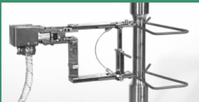
3555 with 50 mm gage length and +20/-10% strain range (bottom cable exit).
