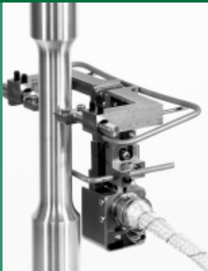
3675 with ±0.15 inch measuring range.
