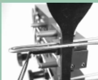
Close-up showing one spring clip that attaches to sample.
