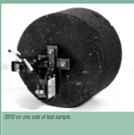
Two 3910 units mounted on asphalt test sample.
