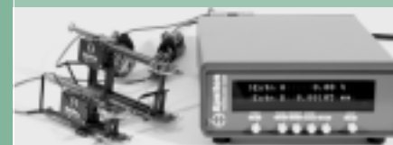
DSM-Plus, two channel version, with 3542 extensometers.
