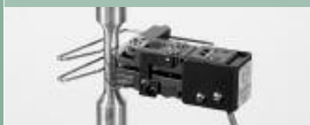
3442 with 0.25" gage length and ±10% strain range.
