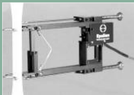
3542 with a 2" gage length and ±25% measuring range.
