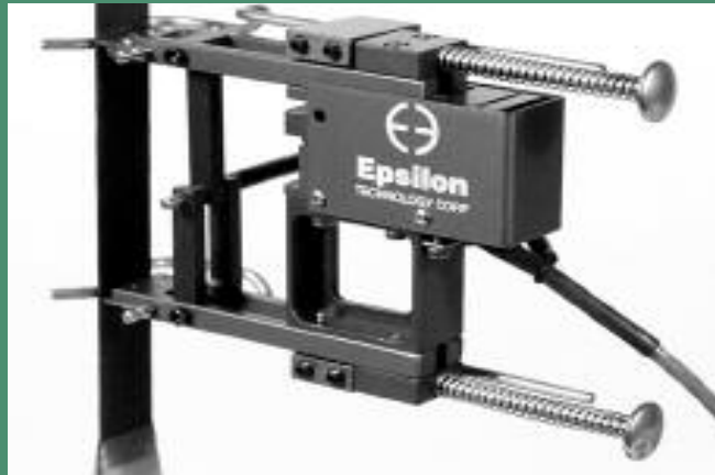
3542 with a 50 mm gage length and ±5% measuring range.
