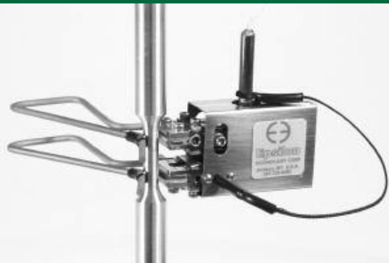
4030 with a 0.5 inch gage length and \pm 5\% measuring ranges.
