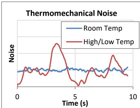
Thermomechanical noise corresponding to elevated temperature or cryogenic tests is wandering noise with a characteristic time interval of ~0.1 to 10 seconds and amplitude that correlates to the test temperature. See [www.epsilontech.com/tech-notes](http://www.epsilontech.com/tech-notes) for help mitigating thermomechanical noise. ([Epsilon TechNote-High Temp Thermomechanical Noise](#) & [Epsilon TechNote - Cryogenic Thermomechanical Noise](#)).
