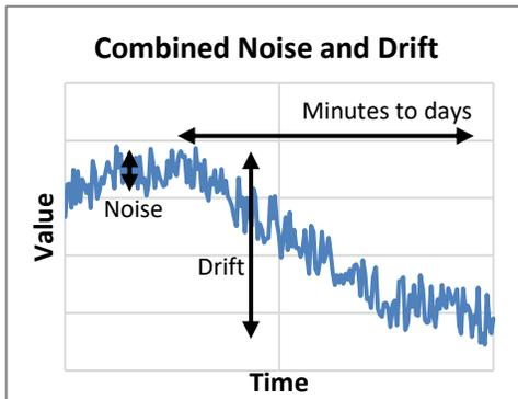
Slowly varying readings with a long characteristic time period (minutes to days) are referred to as *drift* and are often correlated to changes in temperature. Drift can sometimes be much larger in amplitude than noise.
