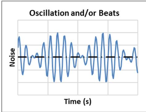
A variety of common causes can result in oscillating, sinusoidal noise, potentially much greater than the typical range. Mechanical vibration, hydraulic noise, and strain control feedback are common causes. Beats (as at left) may or may not be present.
