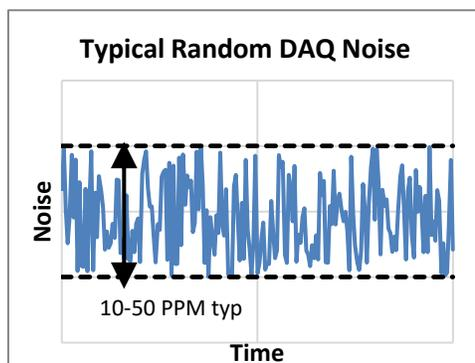
High-frequency / random measurement noise with no visible characteristic frequency, with a constant amplitude over time, which is not related to test temperature, vibration, or test control mode, is usually an indication of the basic measurement resolution of the data acquisition system (DAQ). 10-50 PPM of the range of the extensometer is typical.
