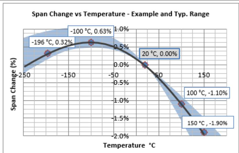
This generic example is typical for strain-gaged devices. A specific curve for any extensometer can be generated by Epsilon during production or calibration service.
