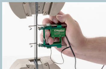
Model 3542 Quick Attach feature enables mounting with one hand
