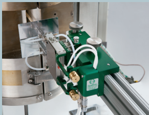
Model 3549 with 25 mm gauge length
