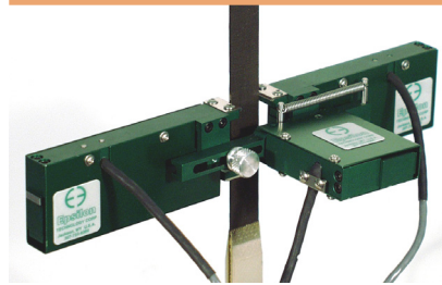
Model 3560 with 25 mm gauge length
