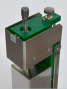
Coarse and fine adjustment knobs for fast and accurate positioning
