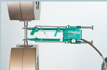
Model 3742 with 25 mm gauge length and +25 mm / -5 mm measuring range
