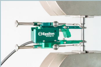
Model 3742 with 25 mm gauge length and +12.5 mm / -5 mm measuring range
