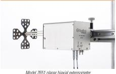
Model 7651 planar biaxial extensometer with tension-tension specimen
