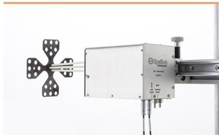
*Model 7651 planar biaxial extensometer with tension-tension specimen*
