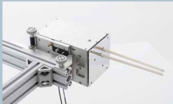
Model 7651 extensometer with 12.5 mm X and Y gauge lengths
