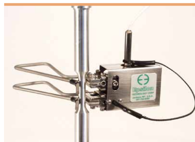
Model 4030 with 0.5 inch gauge length
