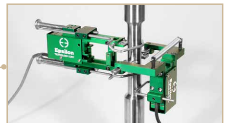
Models 3542 and 3575 extensometers
