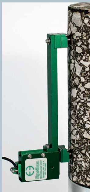
Model 3909-0400 with 4 inch gauge length
