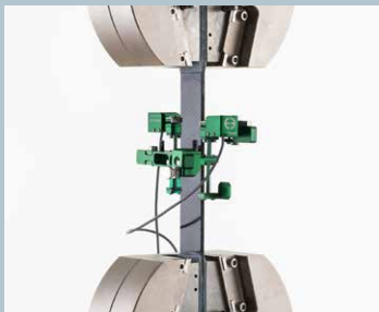
Model 3442AVG extensometer 3442-050M-025M-ST
