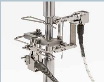
Models 7642 and 7675 extensometers
