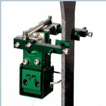
Model 3475-050T-ST with \pm 0.050 inch measuring range
