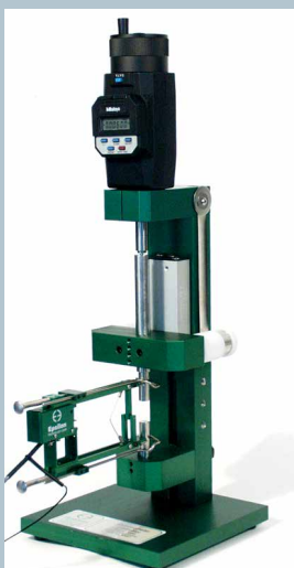
Model 3590 calibrator with Model 3542 axial extensometer
