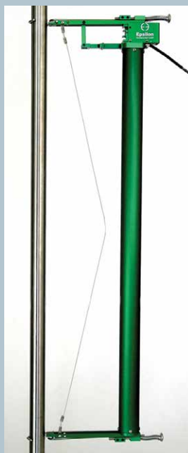
Model 3542L with 500 mm gauge length and +12.5 mm/-6 mm measuring range
