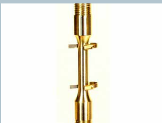
Laser extensometer high temperature clip-on reflectors
