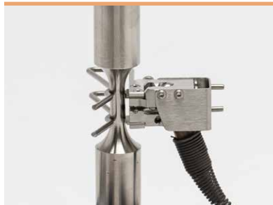
Model 7642-010M-025M extensometer
