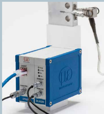
Model 7641 COD gage with signal conditioner
