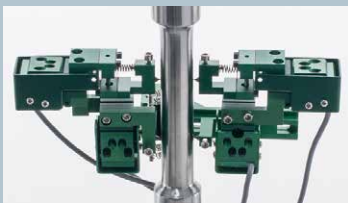
Model 3550 extensometer (back view) 3550-025M-010-002-ST
