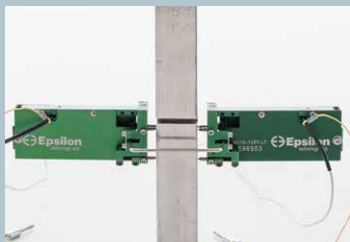
Close-up of the 3 conical contact points used by the Model 4013 extensometer
