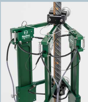
Option for average of three measurements (rebar coupler not shown)
