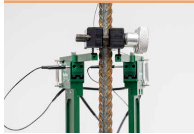
Model 3567 specimen attachment collar with extensometer installed
